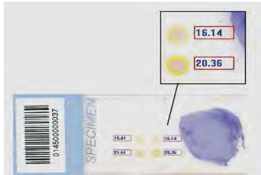
FIGURE 2. Software program screen for measuring stained peptide spot intensity. After subtracting the background level of intensity over irrelevant areas of the slide (not shown), color intensity is measured over the stained peptide spots (contained within the yellow circles). The value, in mean pixel intensity, is depicted in the higher magnification inset. The peptide control spots shown in the inset are not duplicates of each other, but rather serial dilutions. Duplicate peptide controls were printed with a horizontal orientation on the slide.
